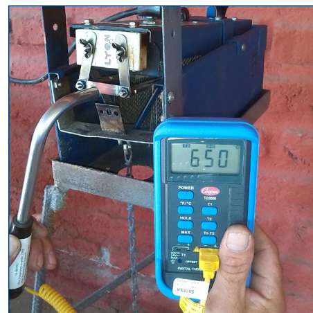
Pyrometer indicating proper blade temperature of 650°C.
