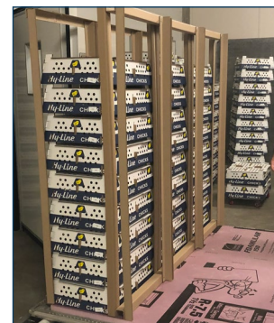
Shipping pallets are constructed of preformed spacers that provide strength and airspace around chick boxes.
